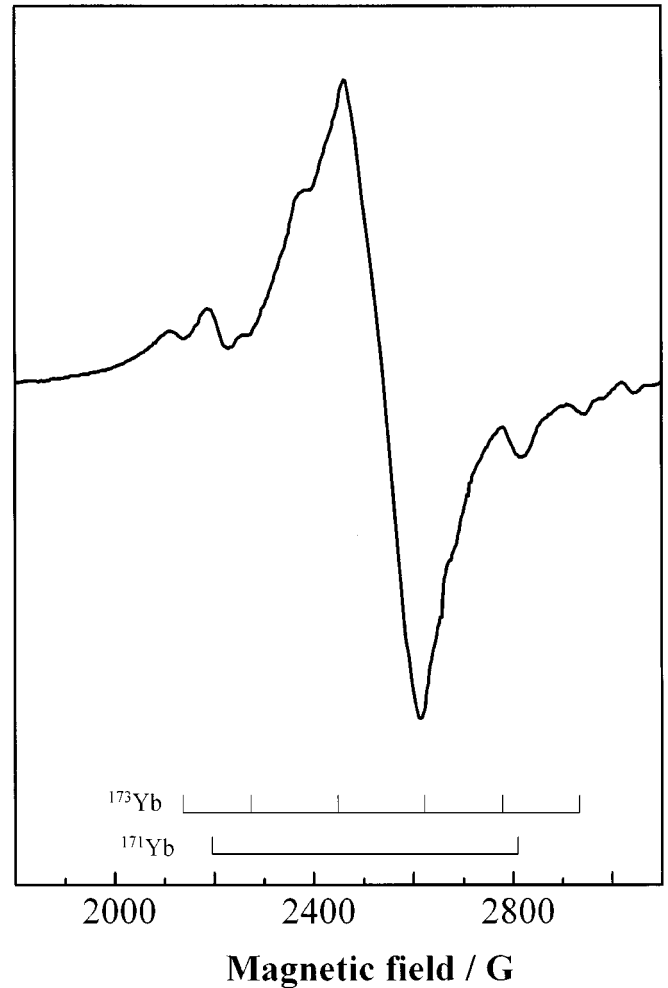
FIG. 5. EPR spectrum of a \text{Yb}^{3+} ion doped in \text{Ba}_2\text{LuTaO}_6 measured at 8 K. Isotropic EPR absorption lines for I = 1/2 and I = 5/2 are depicted with the stick diagram below.
